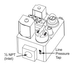
FIGURE 11 - GAS VALVE - REAR
